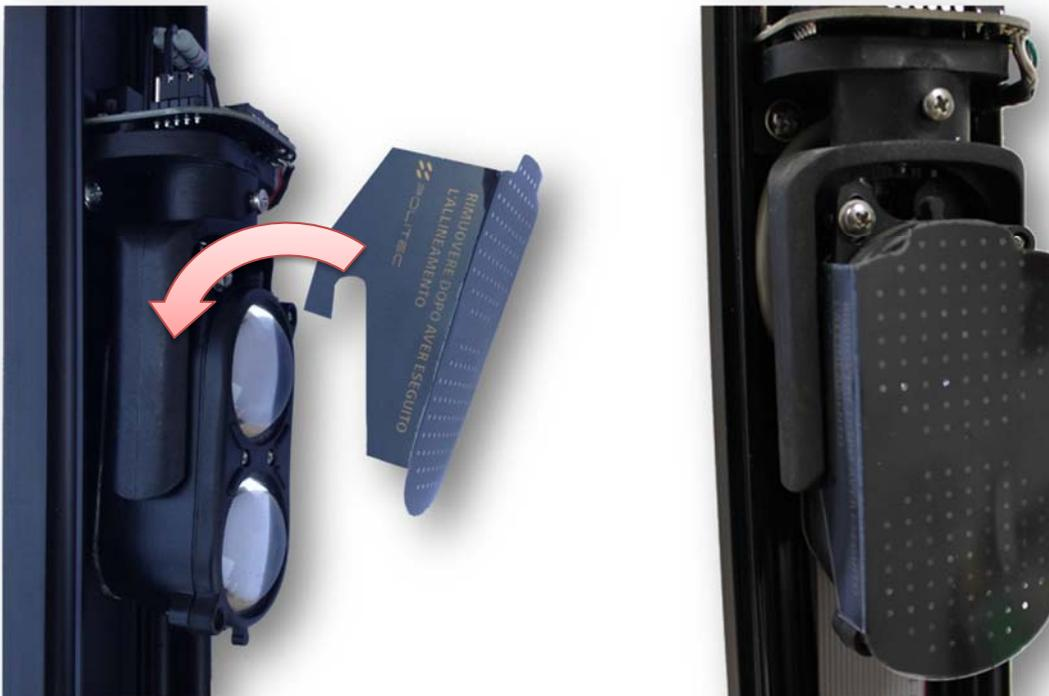
It is enough to apply the filter on TX optic, do not repeat the operation on RX.
